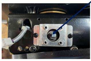
Black mark on magnet denotes the north pole of the magnet. The black mark should be towards the player side of the controller as shown.
