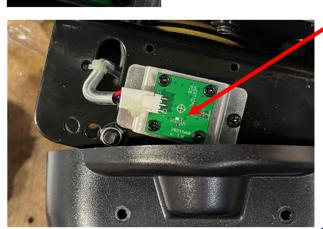
Note the marking on PCB showing north on magnet towards player side of controller
